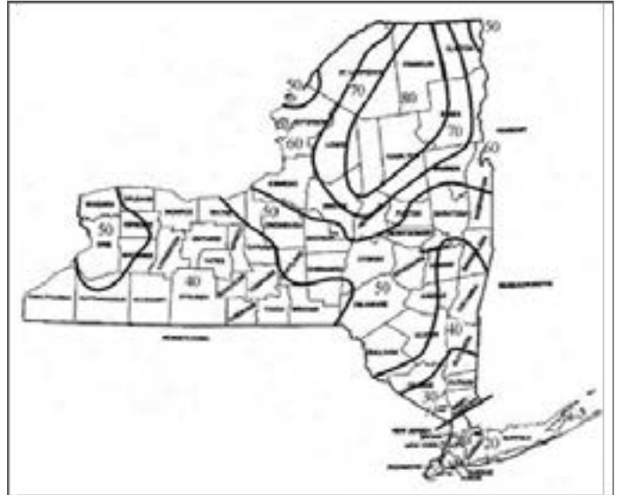
Figure R301.2(5) from NYS Building Standards and Codes 2017 Uniform Code Supplement Ground Snow Loads 5
